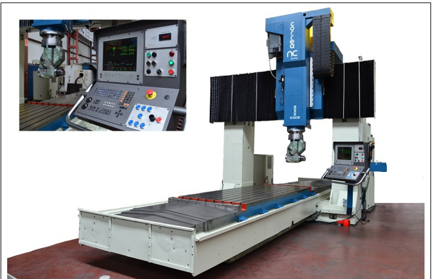
Milling machine CORREA FP40/40
