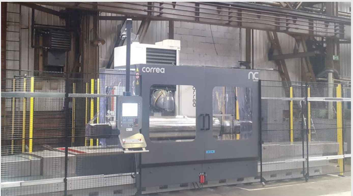
Example of CORREA A30/40 milling machine overhauled with new TNC320 and UDG head
