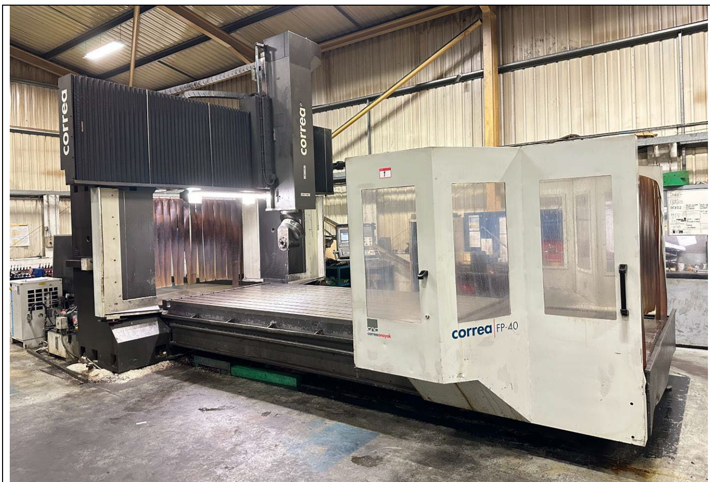
Milling machine CORREA FP40/40 – Before retrofitting
