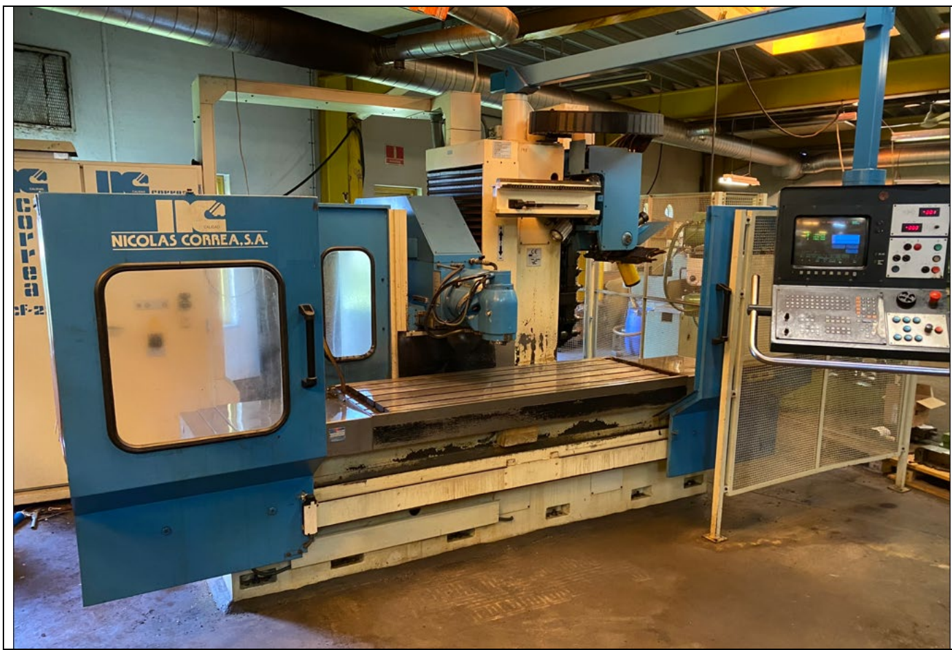
Milling machine CORREA CF22/20 (Before refurbishment process)
