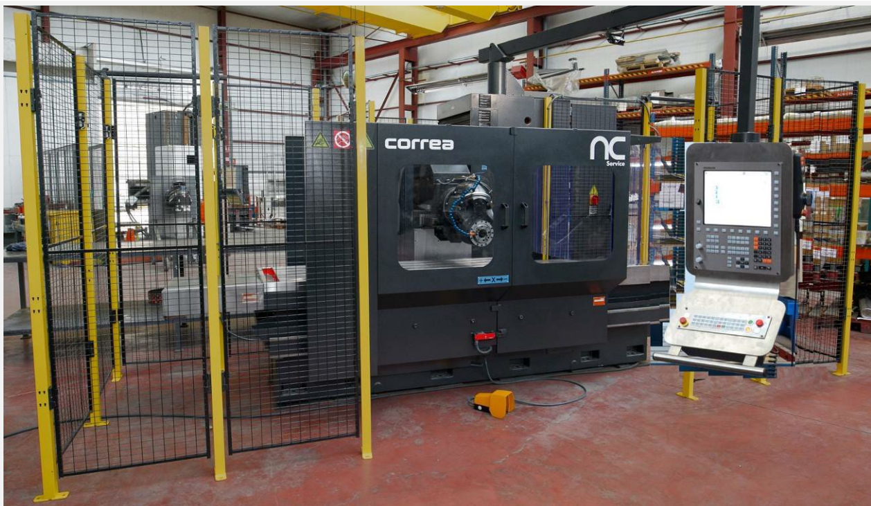
Example of CORREA CF22/20 milling machine refurbished and new HEIDENHAIN TNC-320
