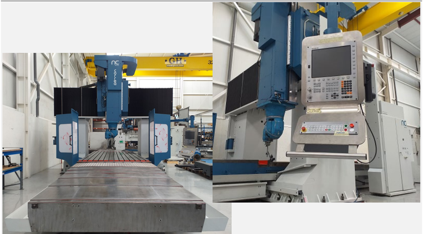
Example of a CORREA FP40 milling machine after retrofitting with new HDH TNC-320
