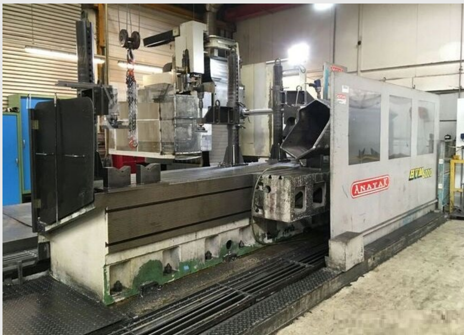
Milling machine ANAYAK HVM-6000 before retrofitting (in origin)
