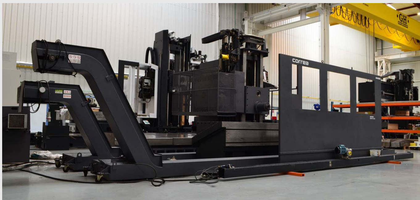
ANAYAK HVM-6000 during mechanical retrofitting process
