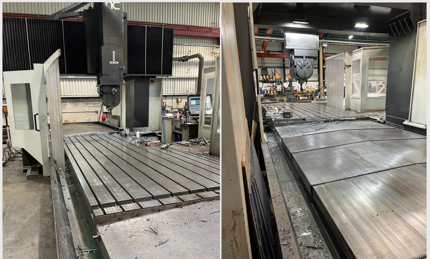
CORREA FP 40/40 milling machine before refurbishment
