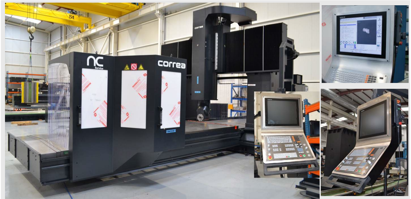
Example of a new HEIDENHAIN TNC-i640 and a CORREA FP 40/40 under retrofitting process
