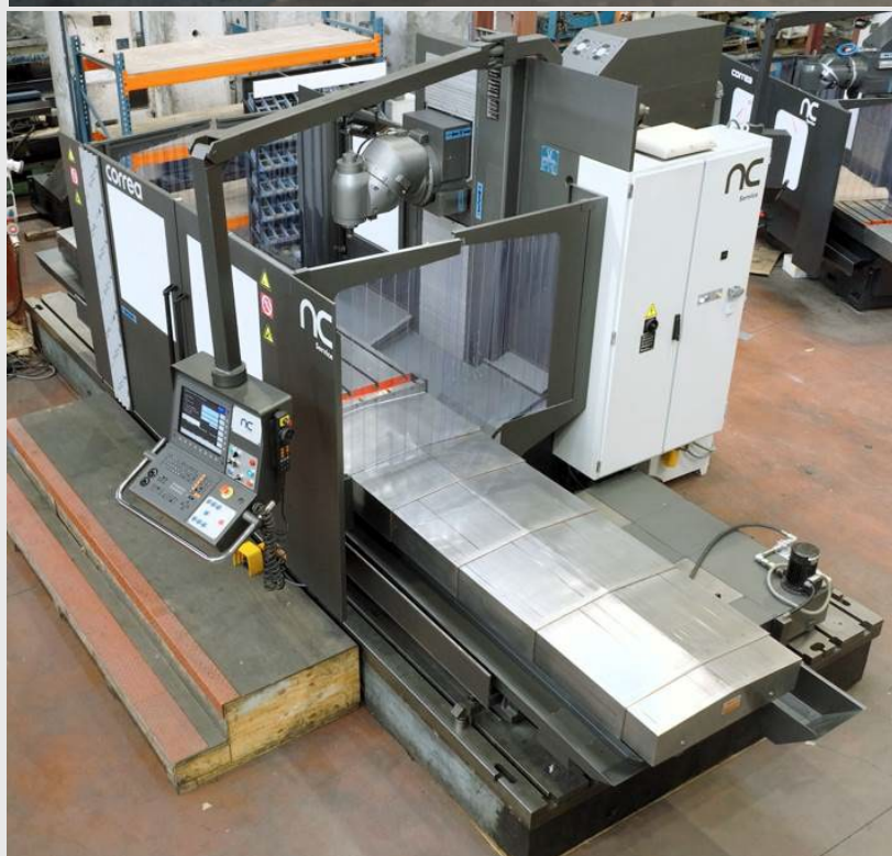
CORREA PRISMA 25 milling machine after mechanical retrofitting
