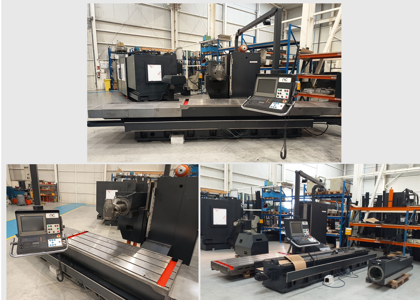
CORREA PRISMA 20 milling machine during retrofitting process at CORREA Service
