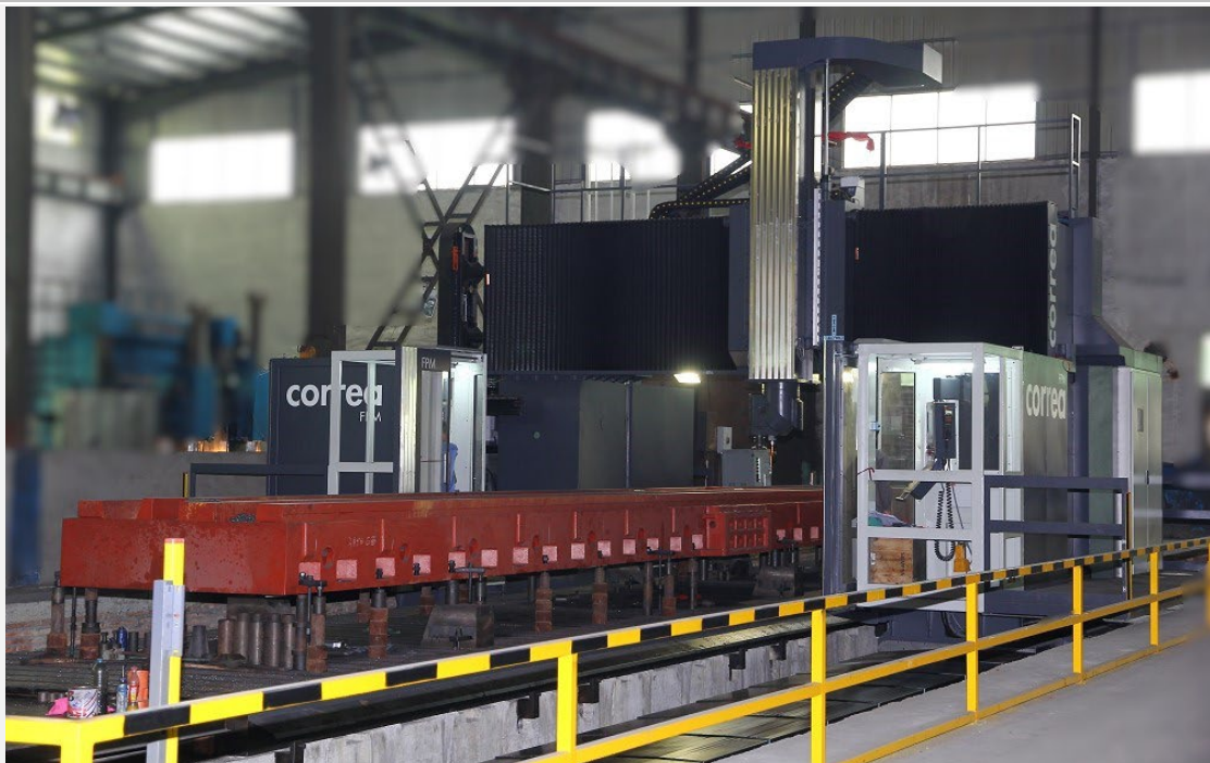
Example of a CORREA FPM50 milling machine after retrofitting process
