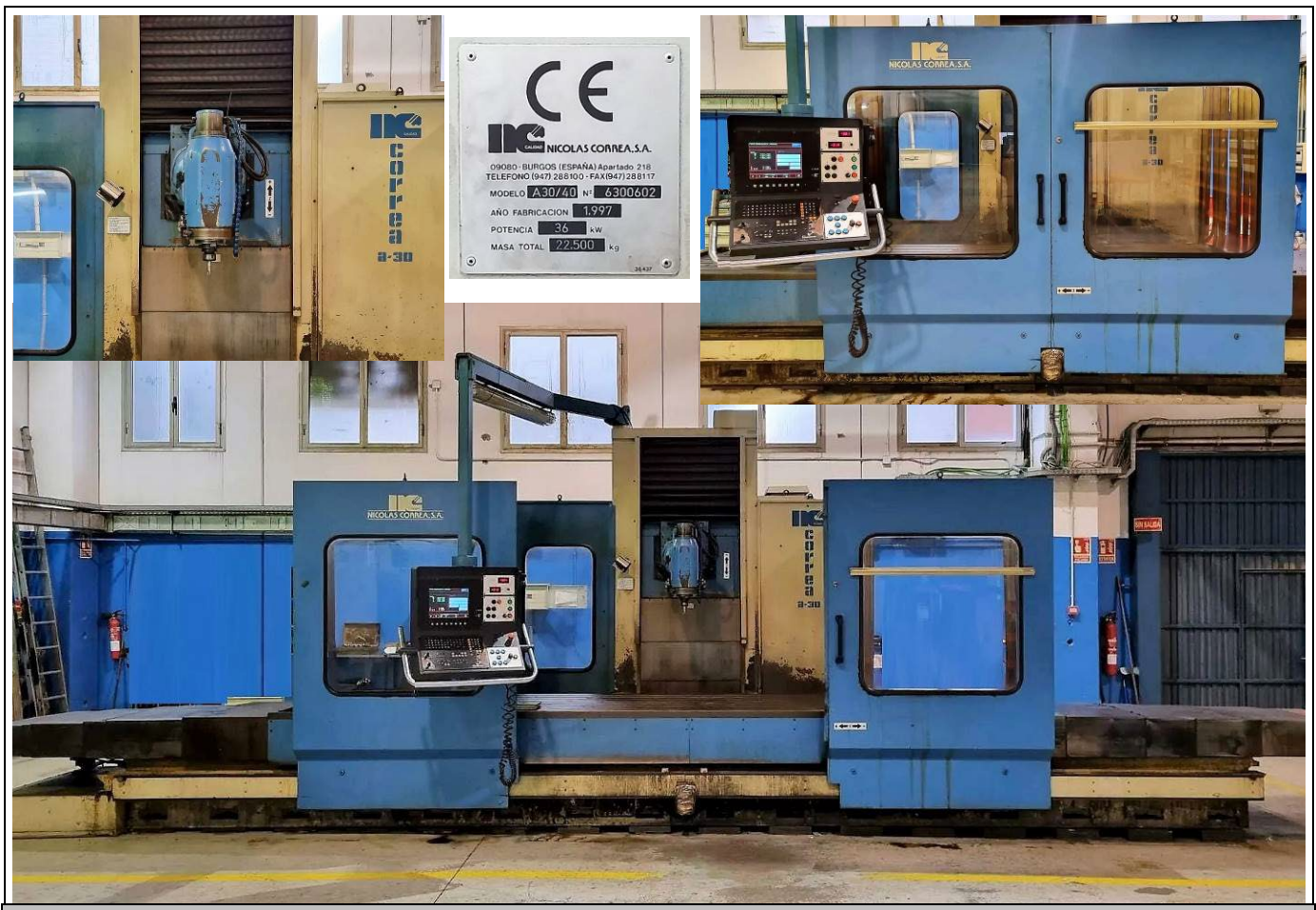
Milling machine CORREA A30/40 (Before refurbishment)
